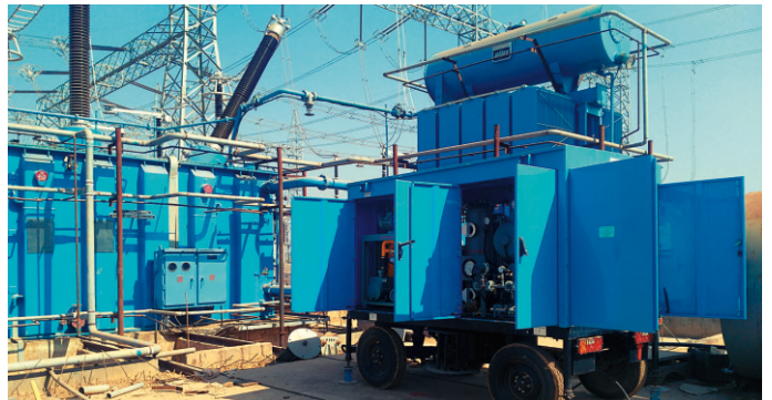
Ultra High Vacuum Transformer Oil Filtration M/c (JHVR 10000X) at BHEL
