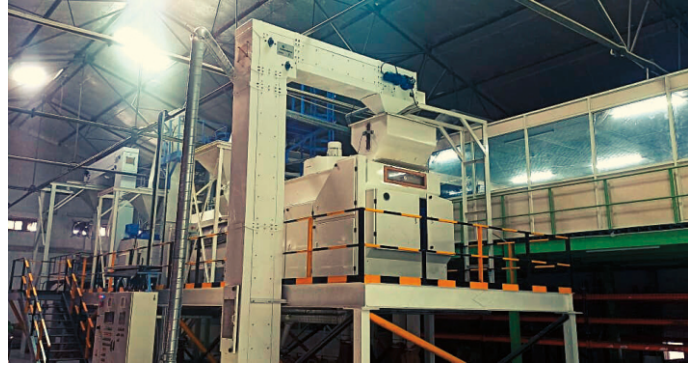
4 TPH Capacity Plant for Grocery & Pulses
